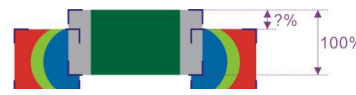
▲ The shift rate is based on component body to the solder pad
