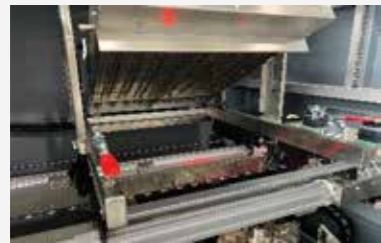
顶部预热 /At the top of the preheating
