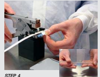
STEP 4 Remove backing paper from splice tape and join cover tapes with splice tape
