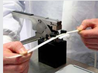
STEP 3 Put depleted reel end into tool, clamp and compress handle of splice tool
