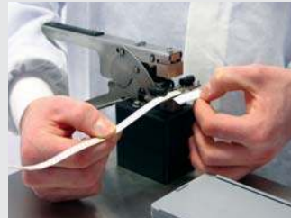
STEP 2 Place new component reel on splice clip
