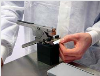
STEP 1 Put SMT Splice Clip into Tape Splicing Tool
